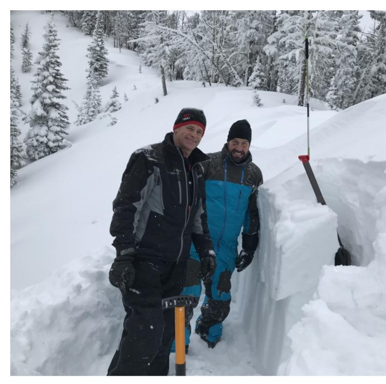
Snow bikers in the northern Gallatin Range found unstable test results on the early December facet layer (12/30). "While snow biking... We dug a snow pit at 9100 ft elevation & discovered a weak layer that propagated at 28 on the ECT test about 18 inches down. The snow below that area was all loosely faceted." Photo: J. Polus
