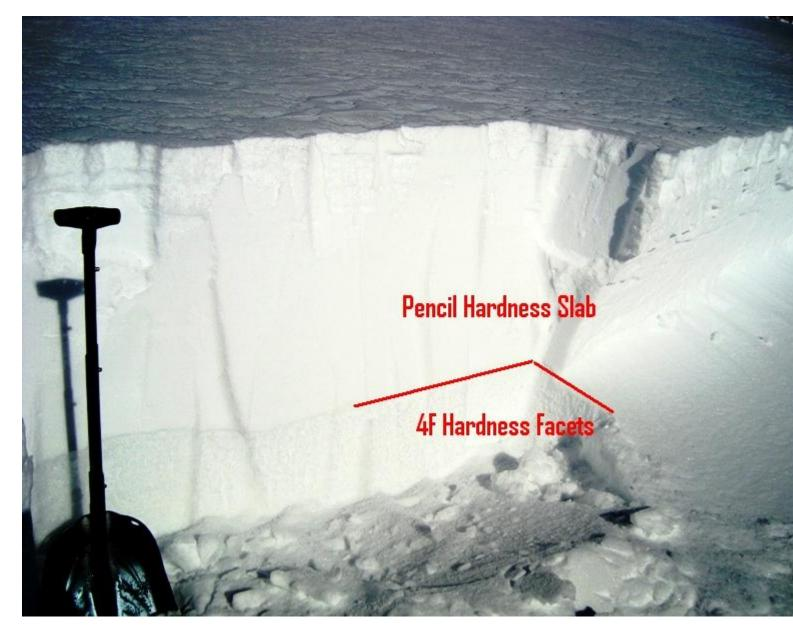
This snowpit was dug in the crown of the slide that a snowmobiler triggered Dec 27. A layer of weak facets could not support the hard slab of wind blown snow plus the rider. The steepest part of the slope was 37 degrees.
