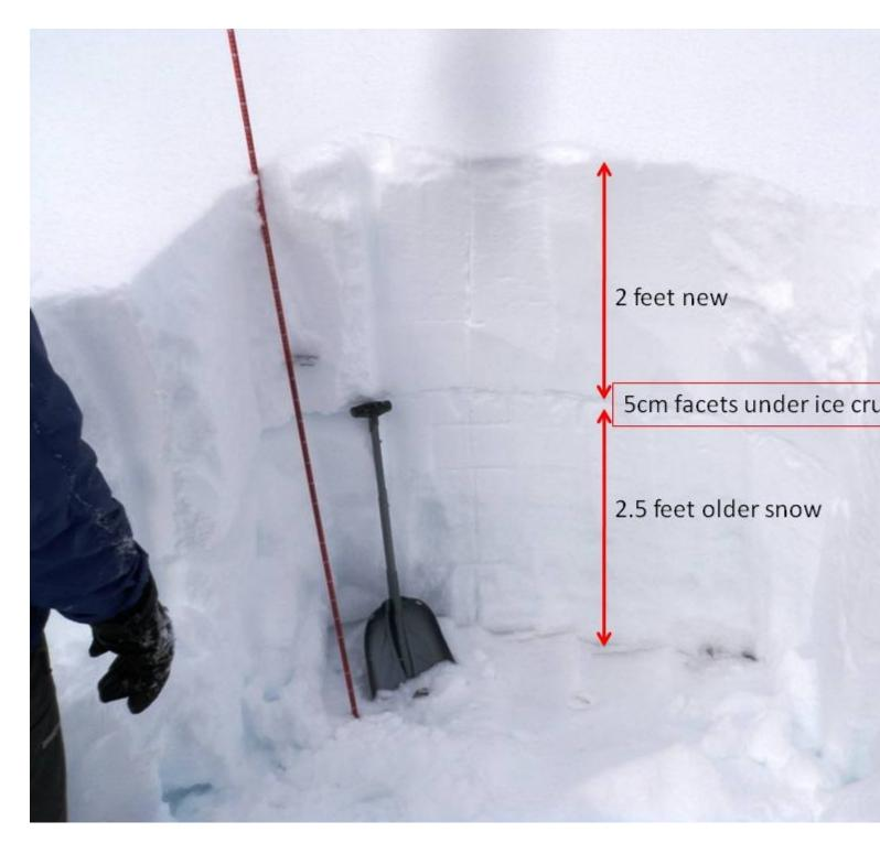
The weak layer stands out easily in the snowpit. The snow depth almost doubled in the last 72 hours which put a huge stress on the weak layer. Photo: Kyle Rott
