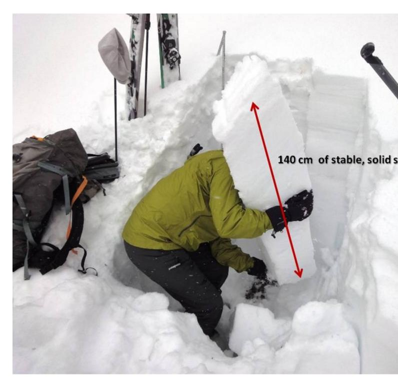
This column of snow would not fracture in my stability tests. Located on a SE facing slope at 7,700 feet on Bacon Rind, it was moist and cohesive. This is the first, real sign of spring I've seen. Photo: GNFAC
