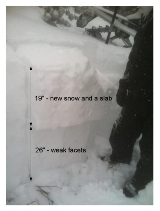
This snowpit in the Cabin Creek area of the Southern Madison Range has a total snowpack depth of almost 4 feet. The bottom 2 feet is all weak, sugary facets and the upper 2 feet is a slab. See the complete snow profile graph <a href="here">here</a>. Photo: B. Radecky
