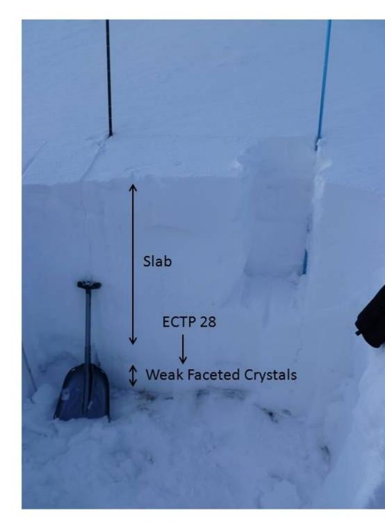
This pit was dug on the flanks of a slide in the 2nd Yellowmule. Strong winds and recent snow heavily loaded north facing slopes. Weak snow near the ground is struggling to support the most recent load. Photo GNFAC
