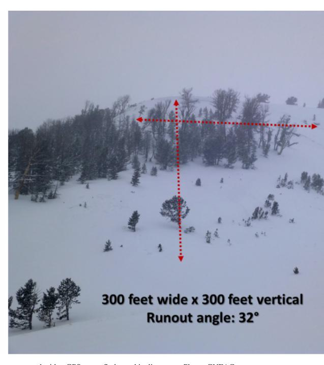
The avalanche size was measured with a GPS, rangefinder and inclinometer. Photo: GNFAC
